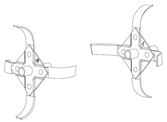
Note: L means left blade, which is different from right blade(R). L and R are engraved on the blade.
